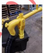
4. Connect black tubing of blasters to "Y" connection.
